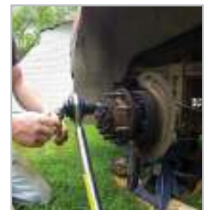
Torque multiplier used for lug nuts
