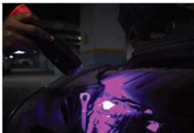
UV light for detecting engine oil leakage, gas leakage, crack in welding jobs in industrial, automotive, HVAC applications
