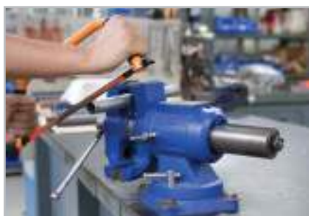
Pipe Jaw can hold pipes with diameter upto 2" (50 mm)
