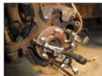
3 Jaw Puller used for removing tyre hub
