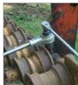
Torque multiplier used on tracks
