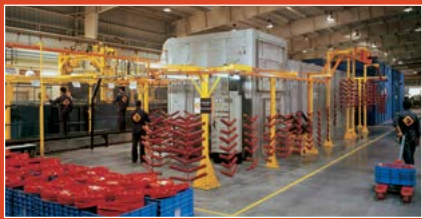
Robotically armed & conveyORIZED double booth powder coating plant with a capacity of 15 million square inch / month
